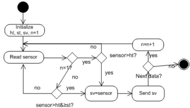
Fig. 5. Basic Principles of TEEN algorithm used in this research [8]
