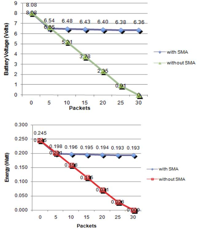
Fig. 7. Battery Voltages and Energy Discharge Rate With and Without SMA on Router Node
