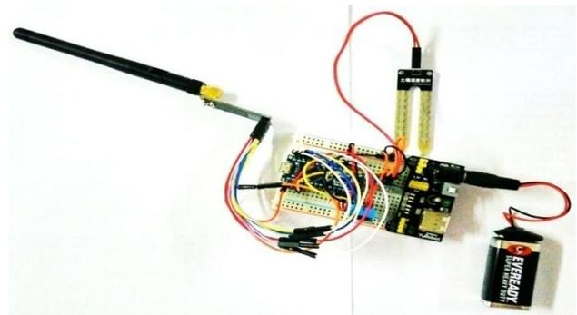
Fig. 3. The Prototype of Sensor Node With 3 Sensors Attached
