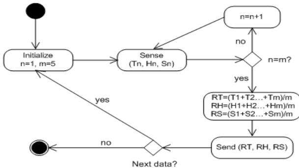
Fig. 4. The SMA Activity Diagram on Sensor Nodes
