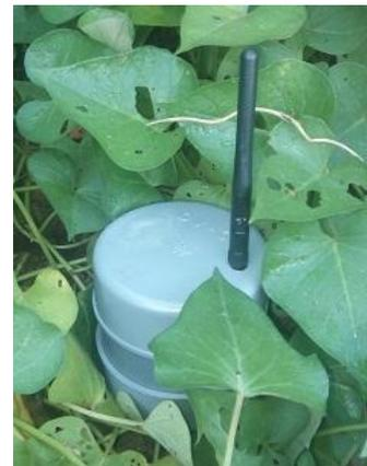
Fig. 1. A Battery Powered Sensor Node For Agriculture Monitoring System
