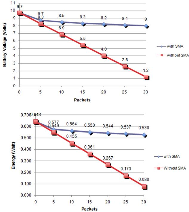
Fig. 6. Battery Voltages and Energy Discharge Rate With and Without SMA on Sensor Node
