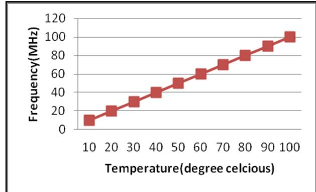
Fig. 2. Temperature of (RO) ring oscillator showing frequency of oscillation linear to temperature.
