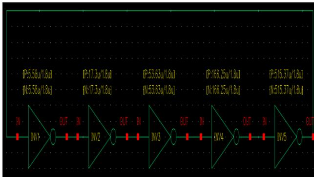
Fig. 10. Schematic ring oscillator with five inverters.
