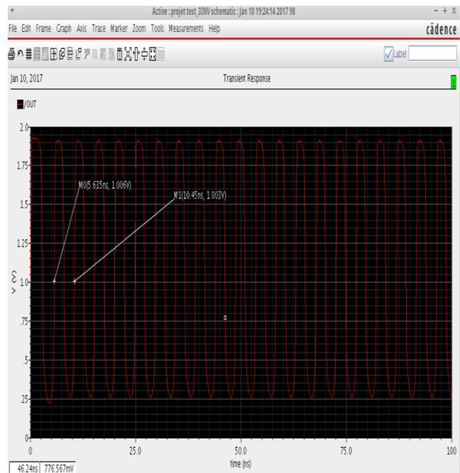
Fig. 9. Display of the period of a ring oscillator with three inverters.
