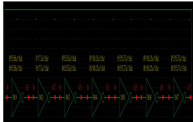
Fig. 12. Schematic ring oscillator with seven inverters.
