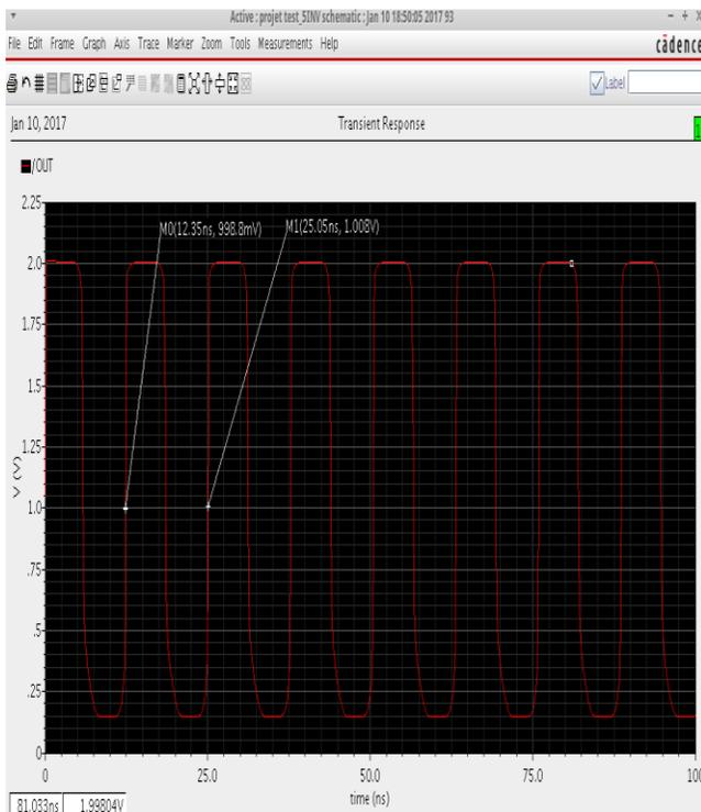
Fig. 11. Display of the period of a ring oscillator with five inverters.
