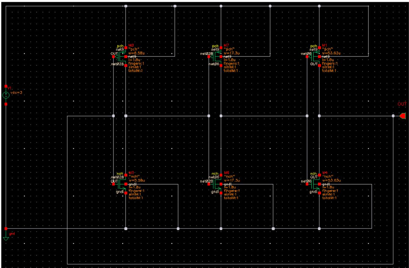
Fig. 6. Schematic of simulation of a ring oscillator with three inverters.
