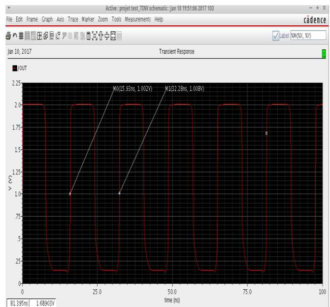
Fig. 13. Display of the period of a ring oscillator with seven inverters.
