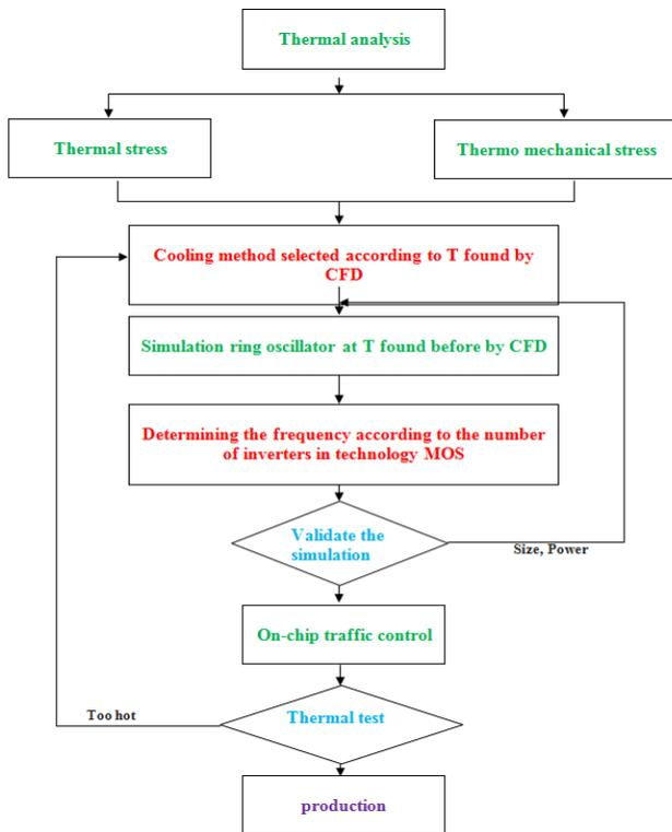
Fig. 1. Methodology for controlling the temperature in the complex system.
