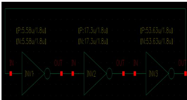
Fig. 7. Schematic ring oscillator with three inverters.
