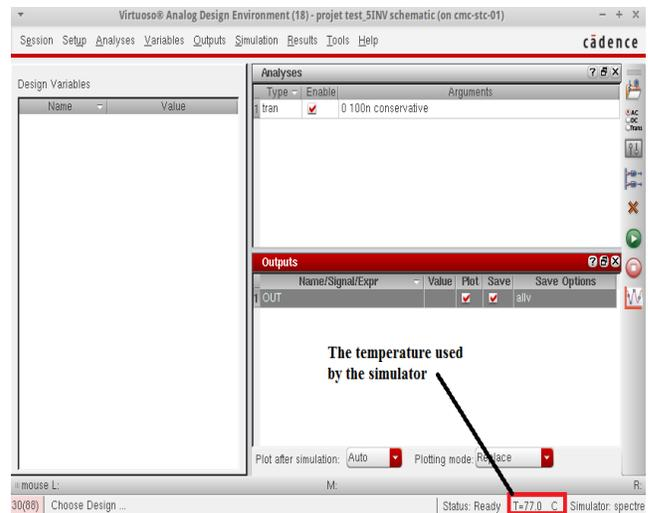
Fig. 8. Virtuoso analog design environment and launch simulations. By simulating this ring oscillator of 3 inverters, we obtain a period of 5.635 ns, corresponding to a frequency of about 208.4 MHz, as shown in Fig. 9.
