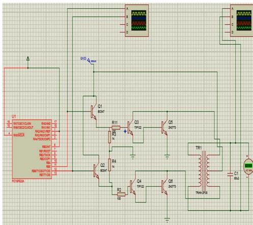
Fig. 5. Simulation model of Inverter
