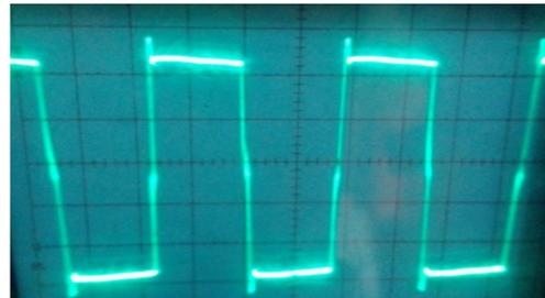
Fig. 8. Output of inverter 1 with load
