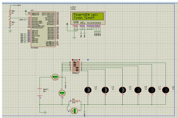
Fig. 10. Simulation Result Showing T1 on only
