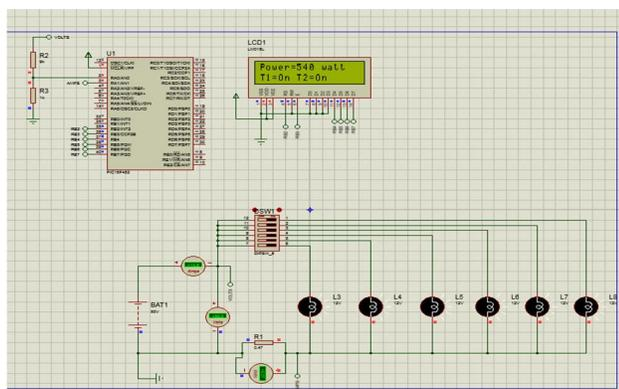
Fig. 11. Simulation Result Showing T1 & T2 both ‘ON’
