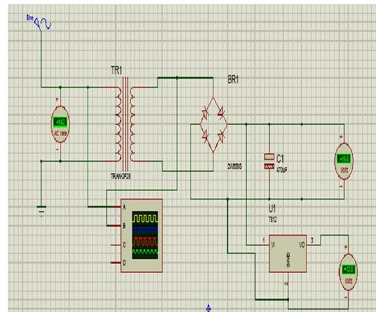
Fig. 3. Simulation Model for AC-DC Converter
