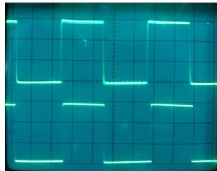
Fig. 9. Synchronized output of 02 inverters
