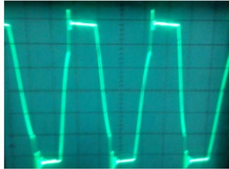
Fig. 7. Output of inverter 1 with no load
